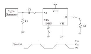
2Vp-p, 10MHz sine wave input signal
